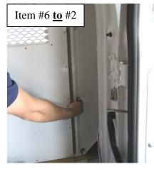
Loosely bolt **Rear Bulkhead Doorframe** (at the door hinge) to **Bench/Wall** assemblies using ½"
